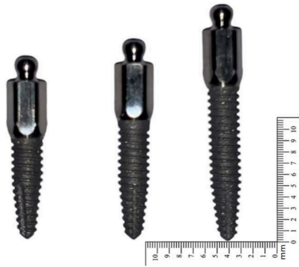
Figure 1. Straight ILZ MDIs from Southern Implants® with a diameter of 2.4 mm. The length of the MDIs was 13 mm ( left ), 10 mm ( middle ), and 8.5 mm ( right ).
